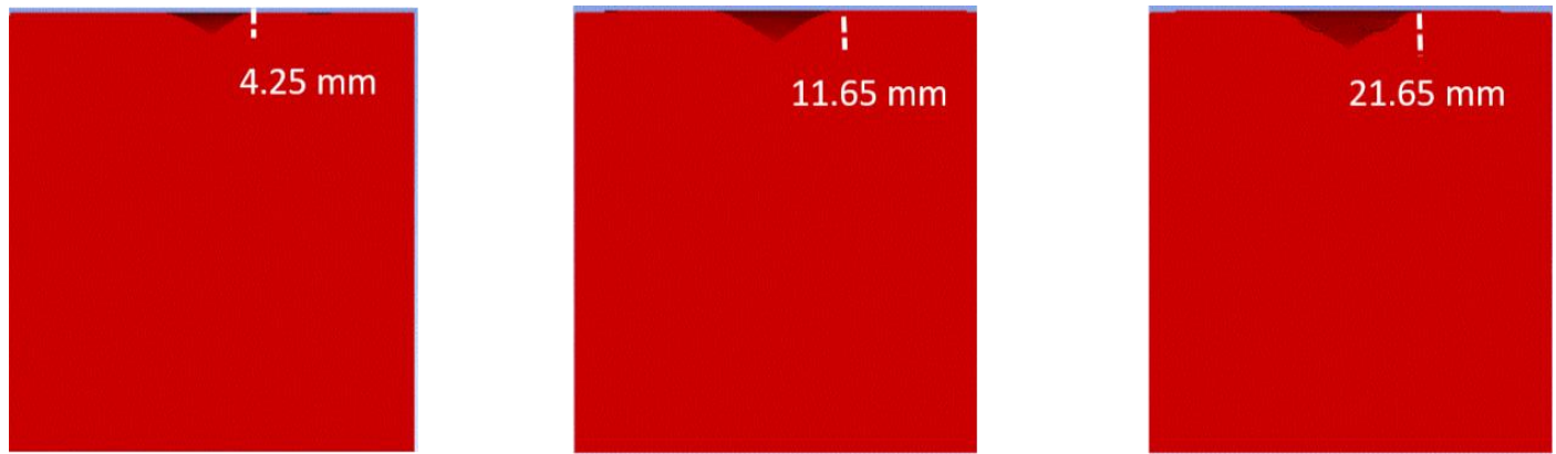
Fig. 5. Cavity formation in the gelatin backing at different time intervals.
